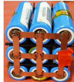
9PS1 Module with 0.5 mm Cell Spacing
