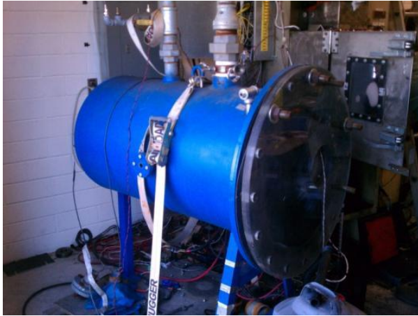
Blast Chamber to Contain Gases and Effluents
