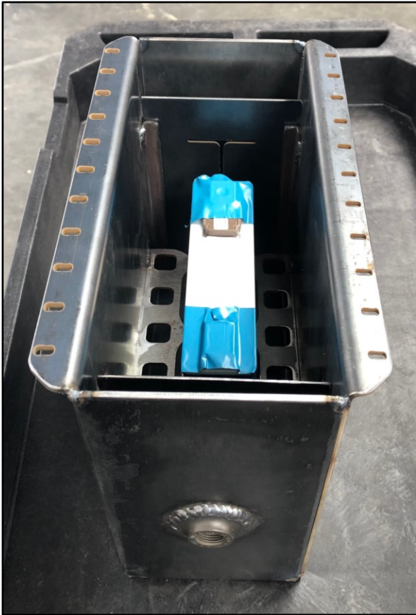
Figure 8: Steel Test Tank with Battery Cell
